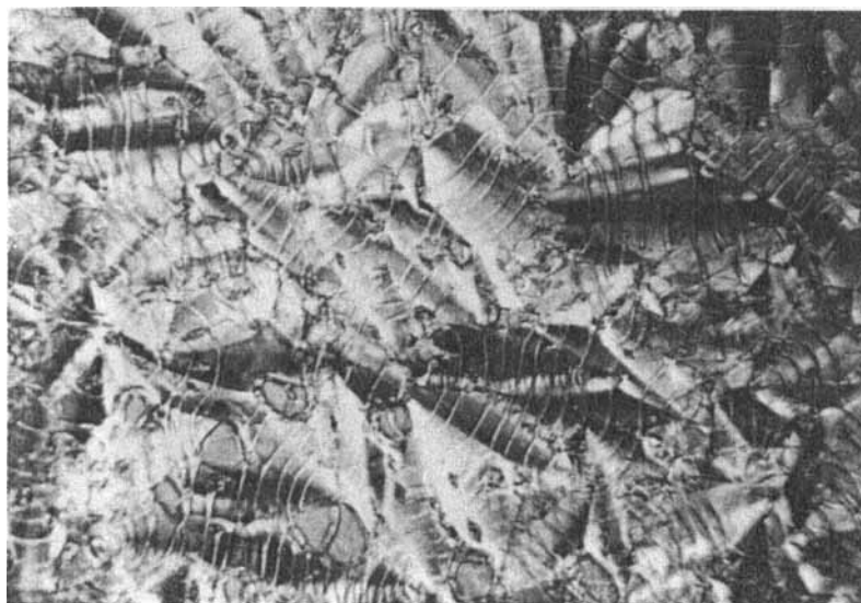
FIGURE 5 Chiral smectic C, fan-shape texture with equidistant lines, for 50% wt A1-6 + 50 % wt B2 T = 55^{\circ}\text{C} ; crossed polarizers (X 250); large pitch ( 10\ \mu\text{m} ). See Color Plate XLII, located in this volume.
